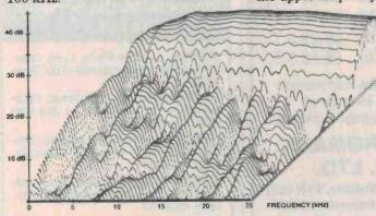
Spectral decay plot to 25 kHz.
