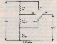
Figure 2. The method of designing this simple switched attenuator is explained in the text.
