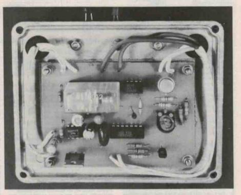
The completed unit was mounted on the lid of a diecast box with a scrap of blank pc substrate underneath as an insulating spacer. The external leads are passed through two grommeted holes.
