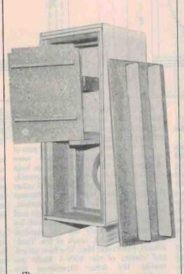
Horizontal braces are added to the internal enclosure baffle and vertical braces to the rear baffle before assembly.
