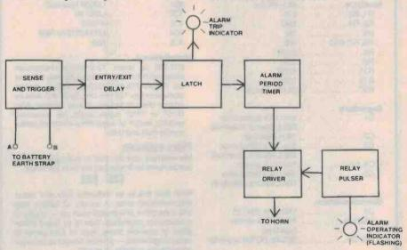
necessary — the project could be con- Figure 1. Block diagram of the ETI-330 car alarm showing the basic functional blocks of the circuit.
