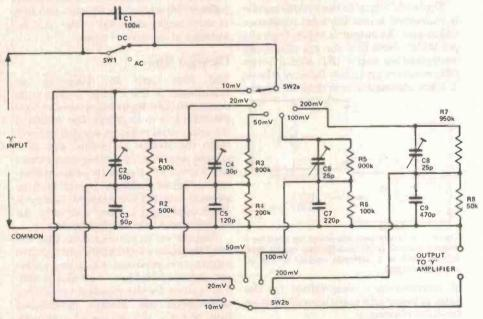
certain pitfalls in using pots in some Figure 4. Section of a typical scope 'Y' amplifier attenuator.
