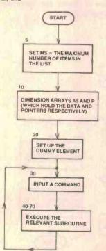
Figure 4. The main program. Flowcharts for the subroutines are given in Figures 5 to 7.
