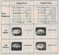
Illustrating how the range of 'pistonic motion', and thus frequency response, is increased by nodal drive.
