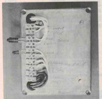
Everything is mounted on the lid of the diecast box and terminations made via a 10-way terminal block mounted on the outside of the lid. Mark each lead, especially polarity where necessary.
