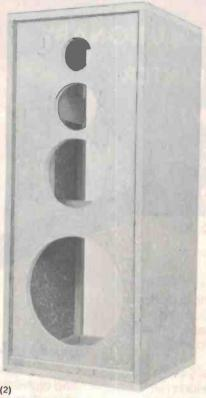
The battens for the midrange-tweeter enclosure are fitted to the box next, followed by the first (larger) front panel.
