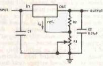
Showing how a three-terminal regulator can be arranged to have an adjustable output. The variable resistor, R 1, here is replaced by a transistor in our regulator circuit below left.
