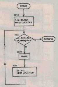
Figure 7. The list routine — the simplest of the three. Note how the addition of a dummy element makes this routine different from Figure 1.
