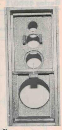
The concrete mix applied to the rear (internal face) of the front baffle.
