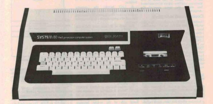
THE SYSTEM 80, as most readers well know by now, is Dick Smith Electronics' answer to the Tandy TRS-80. Early advertising for the DSE machine carried price breakdowns for equivalent systems from both Tandy and DSE, and the System 80 is claimed to be software-compatible with the TRS-80.
